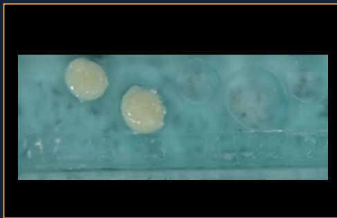
Placing the resin in the portioner holes
