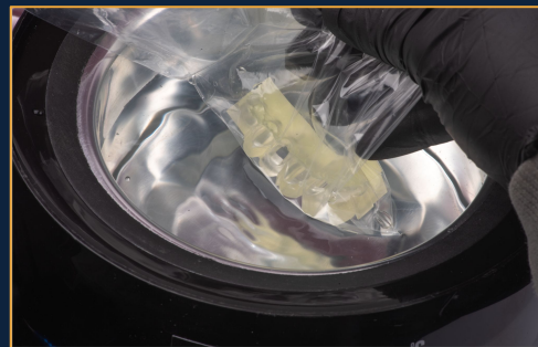
Matrix immersion in heated water (65°C)
